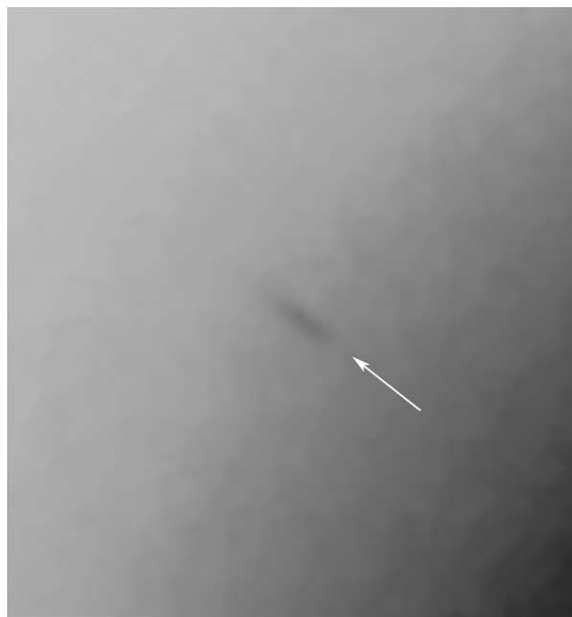
Fig. 10. Magnified region of a diffraction pattern recorded from a longitudinal section of L. hesperus dragline silk. The arrow points to a streak that extends along a vector from the origin. This streak indicates a change in lattice parameter ( \Delta d ) of 0.018 \pm 0.010 \text{ nm} .
